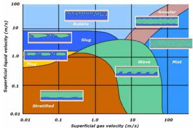
Stratified and stratified wavy flow patterns occur at fairly low liquid and gas velocities. As the gas velocity increases, or if the pipe inclines, then the interface becomes wavy.
