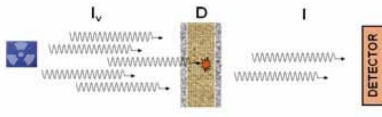
There are two main types of gamma ray attenuation used in multiphase flow meters; single energy and dual energy sometimes referred to as DEGRA (dual-energy gamma ray attenuation). Single energy attenuation uses the high energy gamma ray emitted by a nuclear source to distinguish the gas from the liquid. DEGRA uses both the high and low energy gamma ray emitted to firstly distinguish the gas from the liquid, and then the oil from the water.
