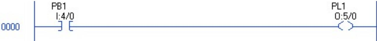
Now let's examine the sequence of events. When you first turn on the PLC, the PB1 pushbutton is off, or false. Therefore, the PL1 output is off. Pressing PB1 will make I:4/0 true, O:5/0 will come on and the light will be energized. It will stay on only as long as you hold the button in.
