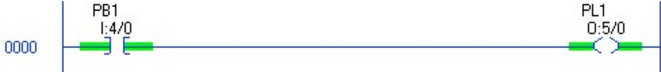
One nice feature of Allen-Bradley PLCs is that you can document each bit in the program. In the example above, “INPUT1” is somewhat meaningless on its own. After you add the descriptive text “Start Motor PB1”, things make more sense.
