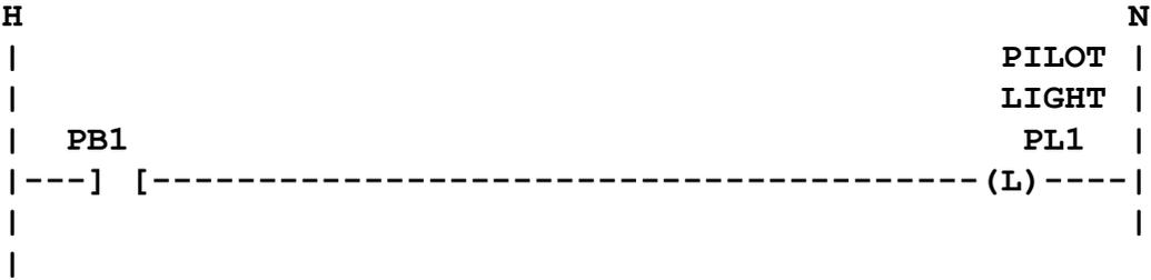
Now let's do the same thing in an SLC. To duplicate the hardwired circuit on a PLC, you would wire the switch PB1 to input I:4/0 and wire the light PL1 to output O:5/0.
